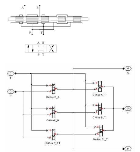
The Orifice with Variable Area Round Holes blocks have been used as a variable orifice in this model. Port T1 corresponds to an intermediate point between ports P and T.
